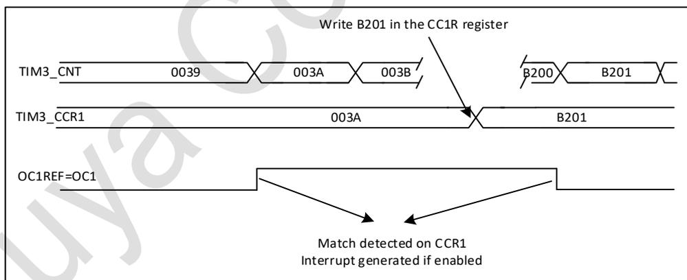
Figure 17-28 Output compare mode, toggle on OC1
