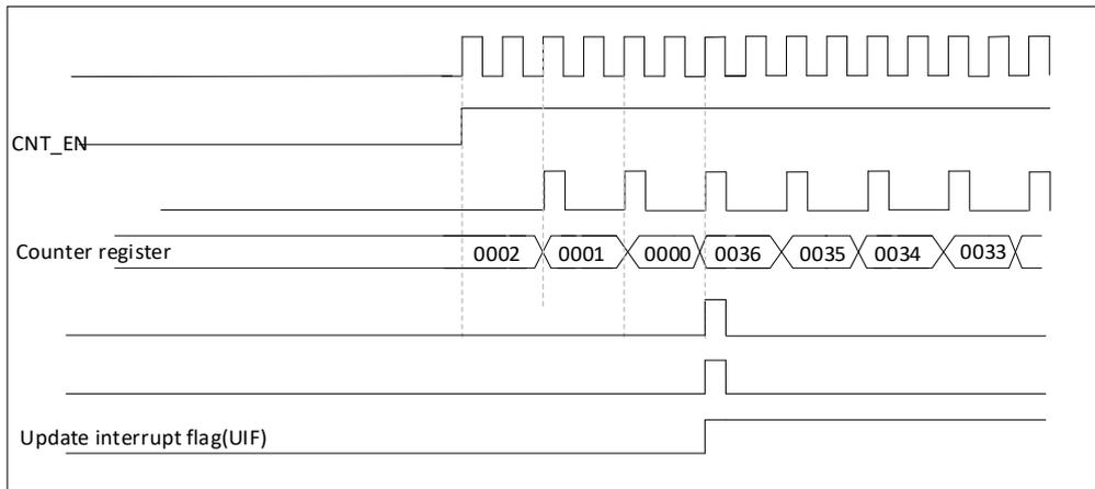
Figure 16-11 Counter timing diagram, internal clock divided by 2
