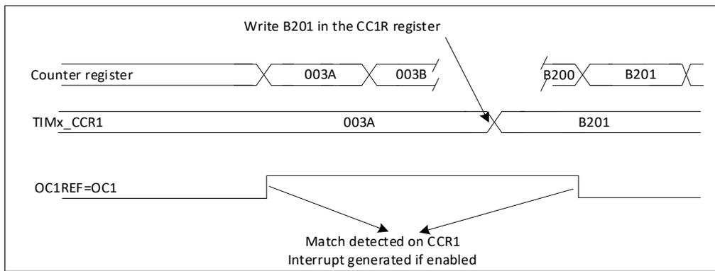
Figure 16-33 Output compare mode, toggle on OC1.
