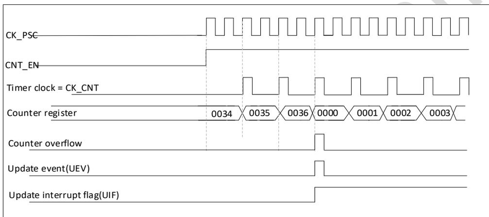
Figure 16-5 Counter timing diagram, internal clock divided by 2
