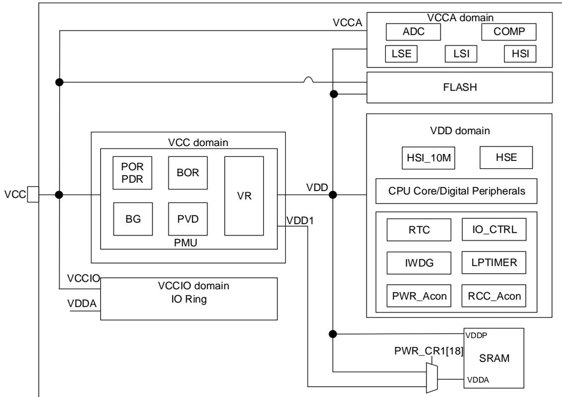
Figure 5-1 Power block diagram
