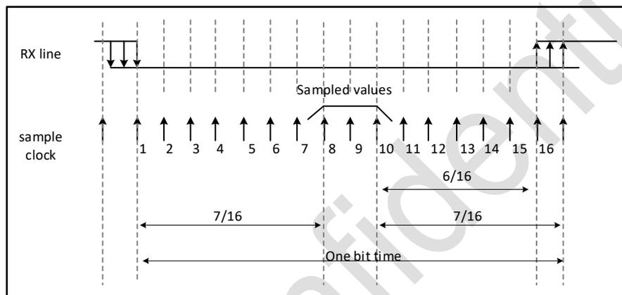
Figure 25-6 Data sampling for noise detection
