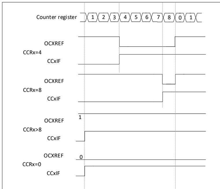
Figure 19-16 Edge-aligned PWM waveforms (ARR = 8)
