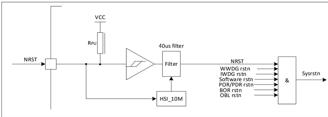
Figure 7-1 Simplified diagram of the reset circuit
