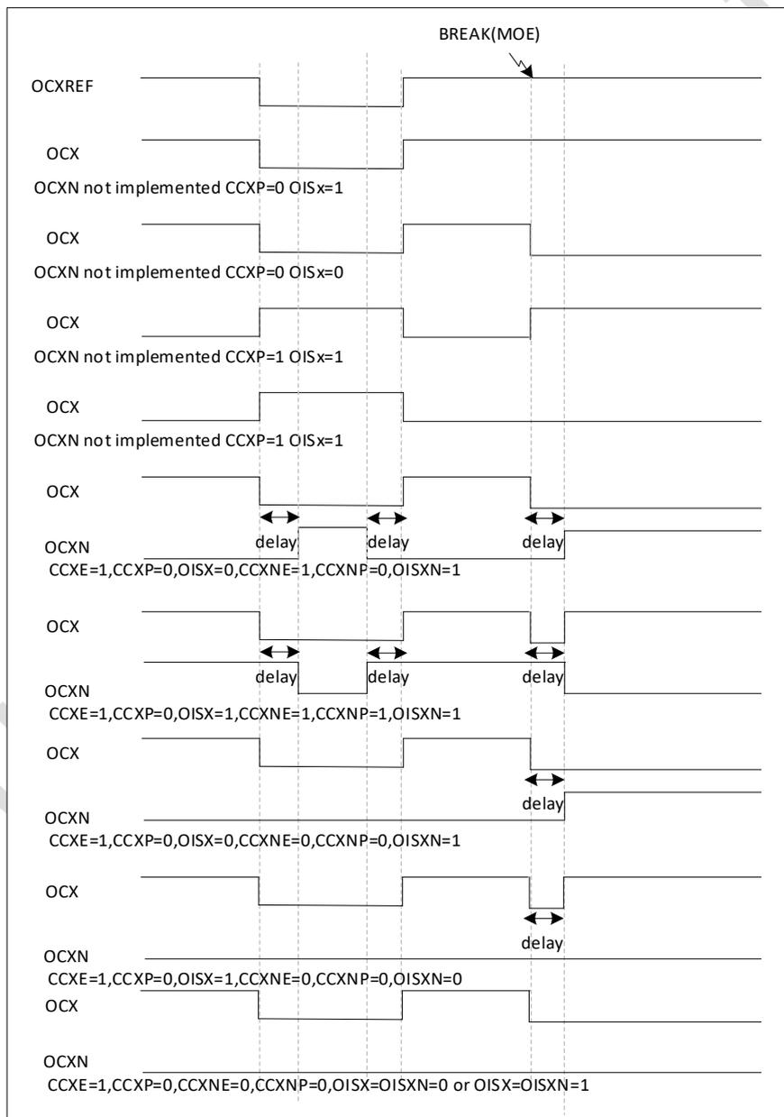
Figure 19-20 Output behavior in response to a break
