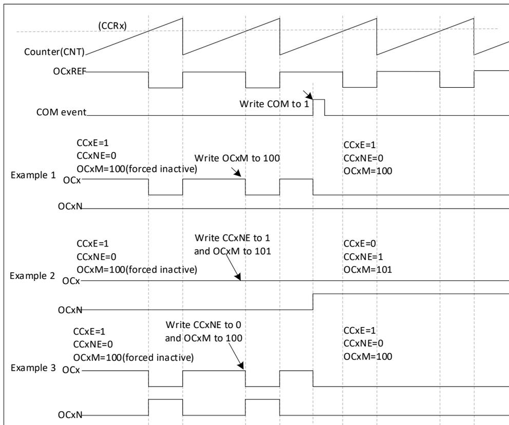
Figure 16-42 6-step generation, COM example (OSSR = 1)
