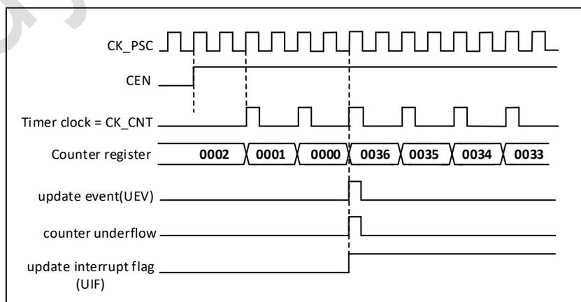
Figure 17-11 Counter timing diagram, internal clock divided by 2
