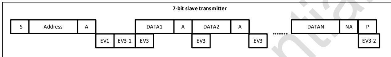
Figure 24-3 Transmission sequence diagram from the sender
