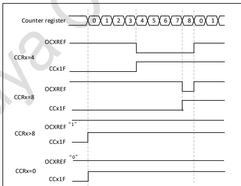
Figure 17-29 Edge-aligned PWM waveforms (ARR = 8)
