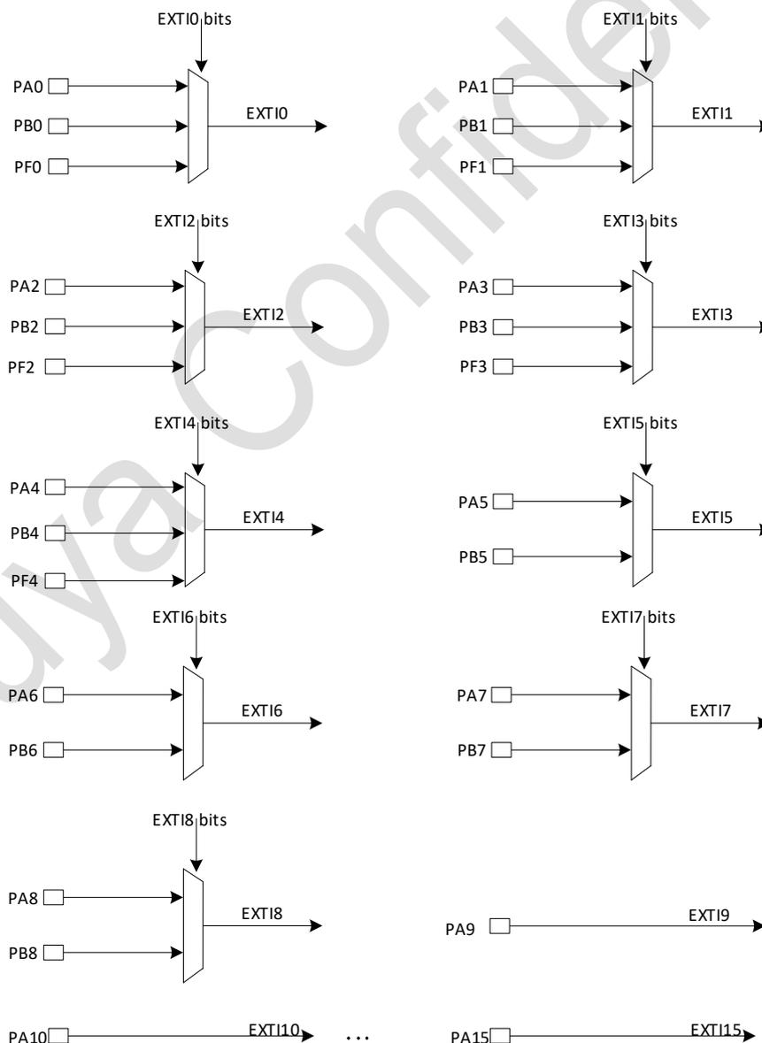
Figure 12-2 External interrupt/event GPIO mapping
