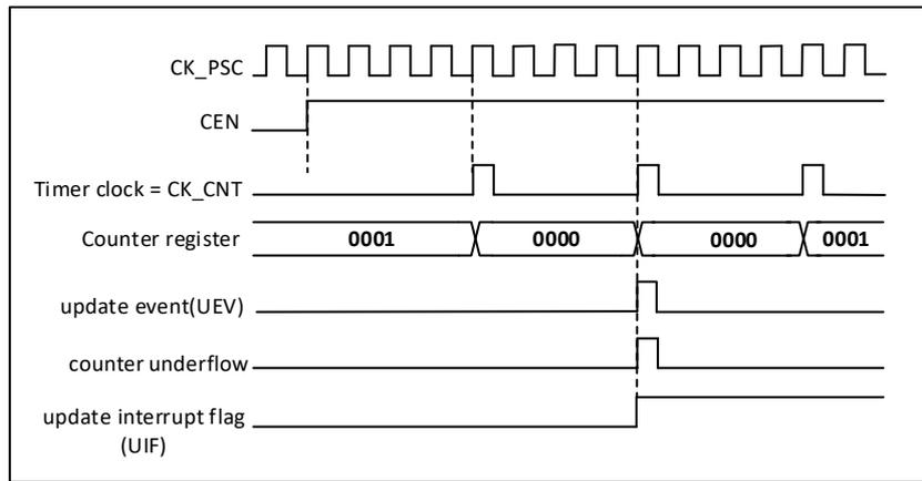
Figure 17-12 Counter timing diagram, internal clock divided by 4
