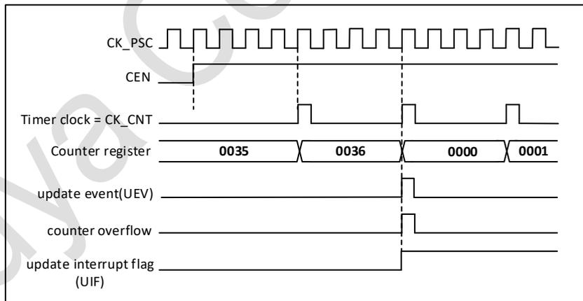
Figure 17-6 Counter timing diagram, internal clock divided by 4
