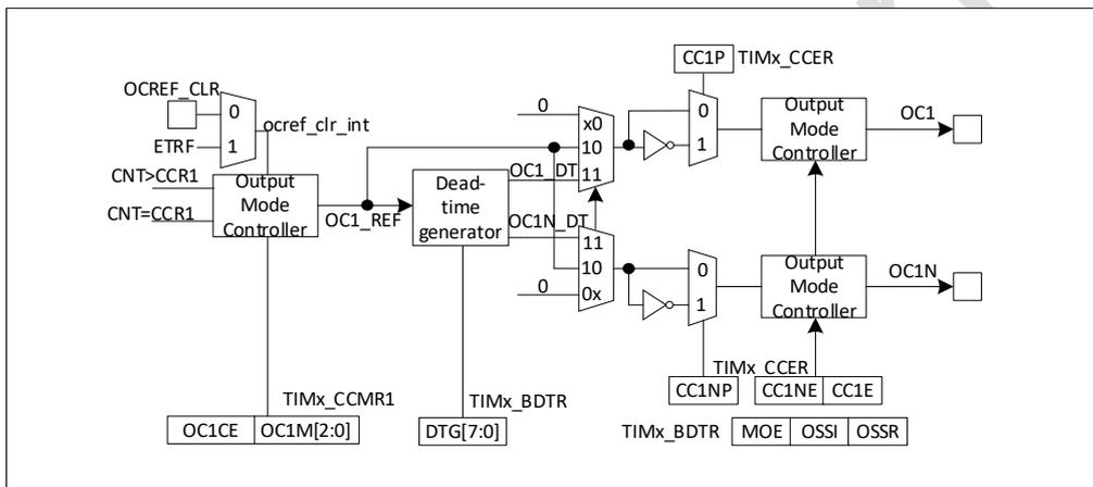
Figure 16-29 Output stage of capture/compare channel (channel 1 to 3)
