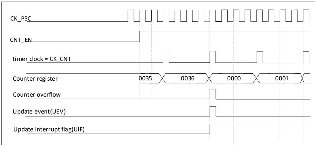
Figure 18-6 Counter timing diagram, internal clock divided by 4
