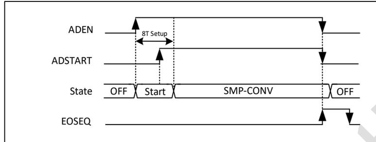
Figure 14-2 Enabling/disabling the ADC
