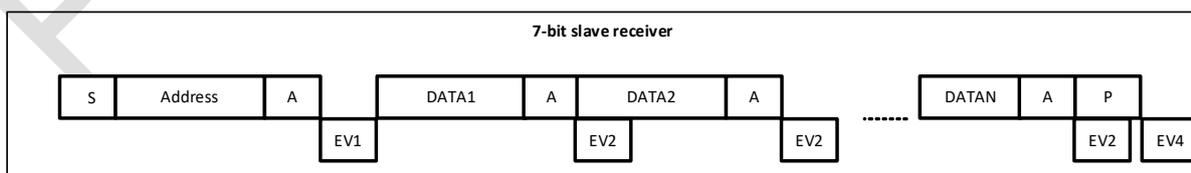
Figure 24-4 Slave receiver transmission sequence diagram
