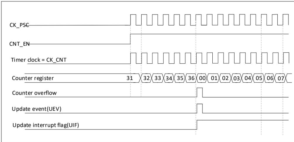
Figure 16-4 Counter timing diagram, internal clock divided by 1
