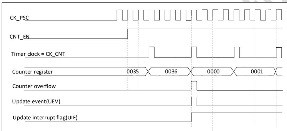
Figure 19-6 Counter timing diagram, internal clock divided by 4
