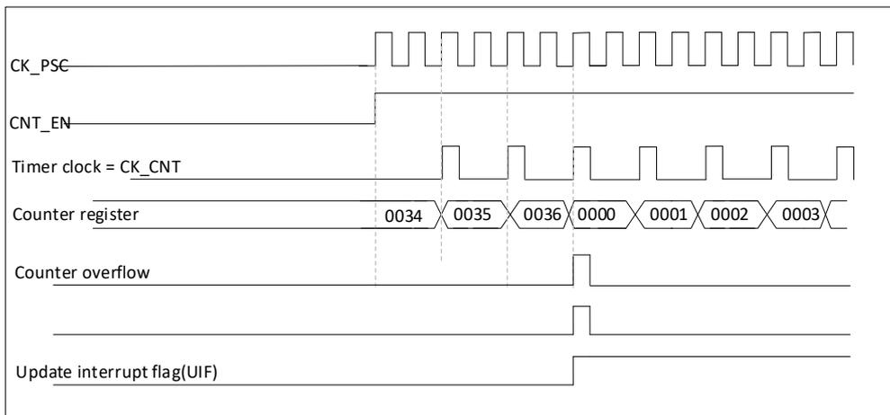
Figure 19-5 Counter timing diagram, internal clock divided by 2
