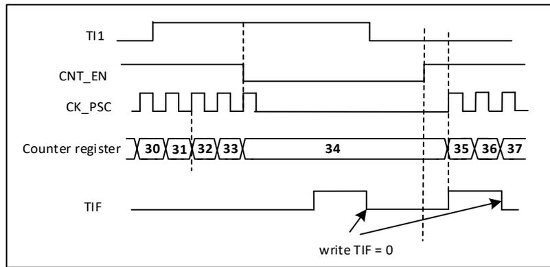
Figure 17-35 Control circuit in gated mode
