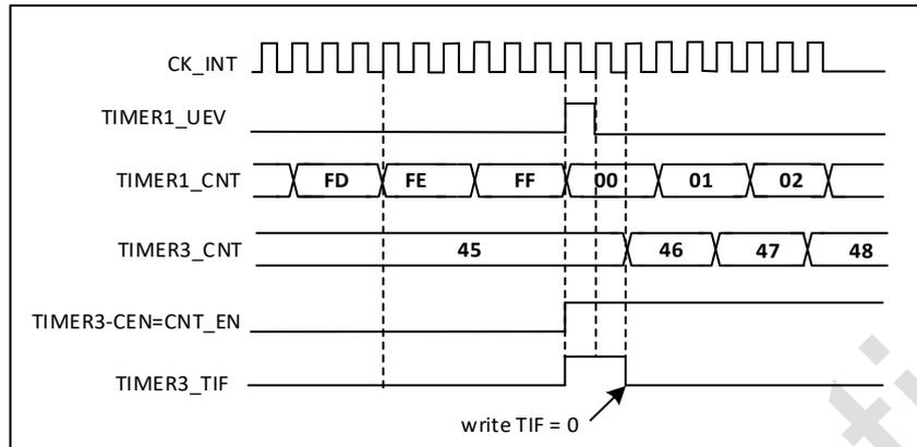
Figure 17-41 Triggering timer 3 with update of timer 1
