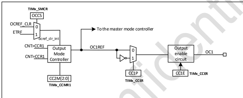
Figure 17-26 Output stage of capture/compare channel (channel 1)
