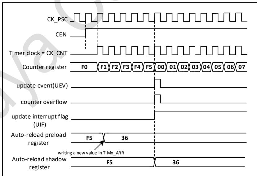
Figure 17-9 Counter timing diagram, Update event when ARPE = 1 (TIM3\_ARR preloaded)
