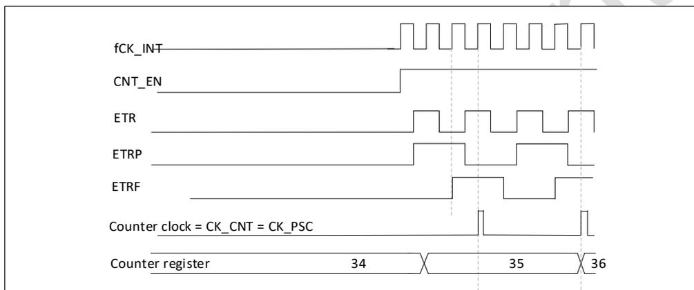
Figure 16-26 Control circuit in external clock mode 2
