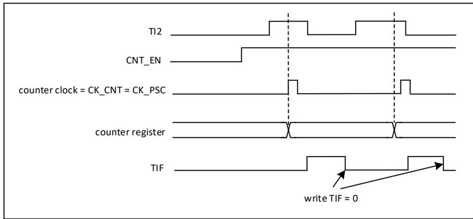
Figure 17-23 Control circuit in external clock mode 1
