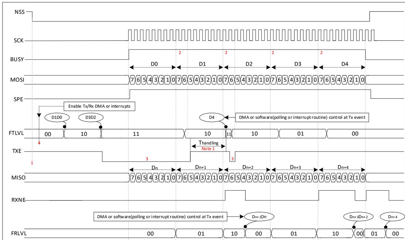
Figure 26-10 Master full-duplex communication diagram(bit frame = 8, FRXTH = 0)
