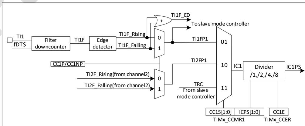
Figure 16-27 Capture/compare channel (example: channel 1 input stage)
