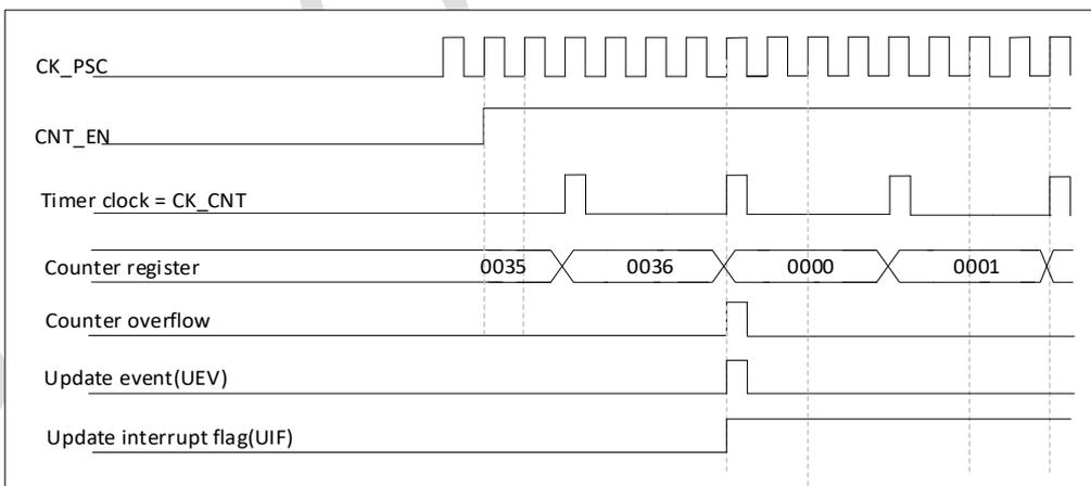
Figure 16-6 Counter timing diagram, internal clock divided by 4
