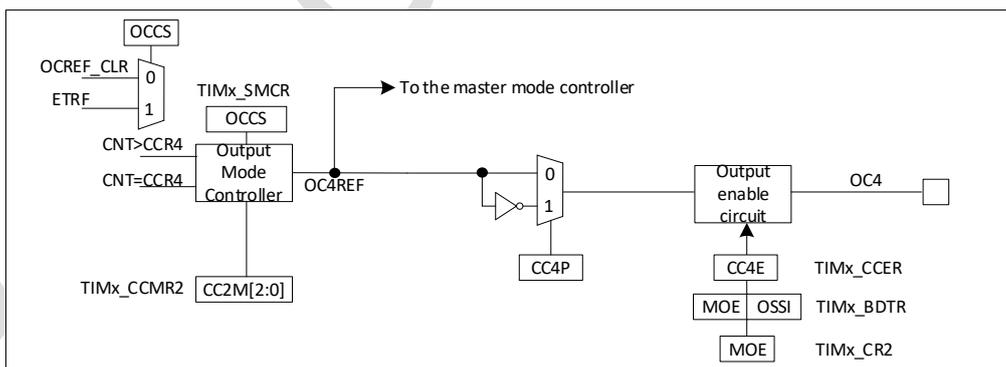
Figure 16-30 Output stage of capture/compare channel (channel 4)
