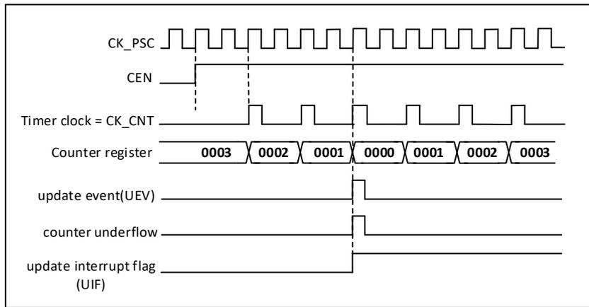
Figure 17-16 Counter timing diagram, internal clock divided by 2
