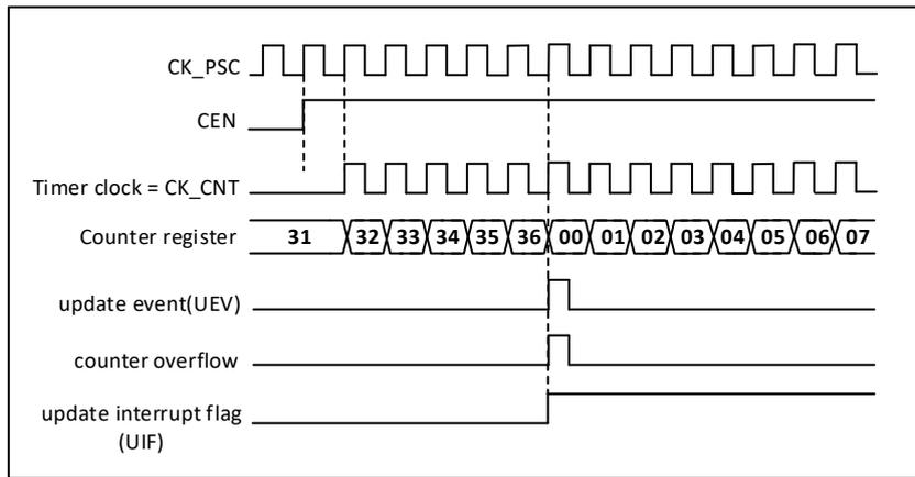
Figure 17-4 Counter timing diagram, internal clock divided by 1
