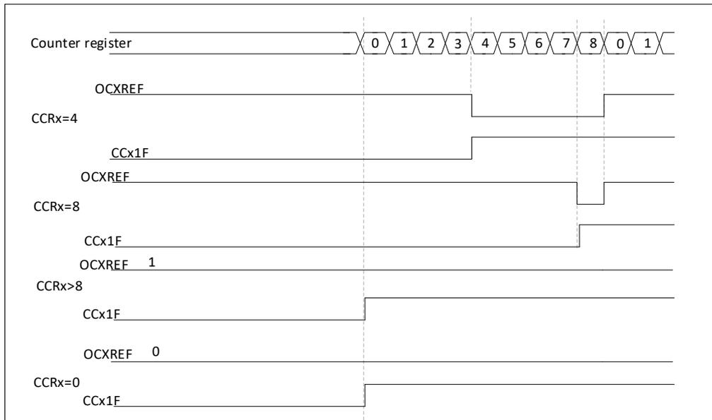
Figure 16-35 Edge-aligned PWM waveforms (ARR = 8)
