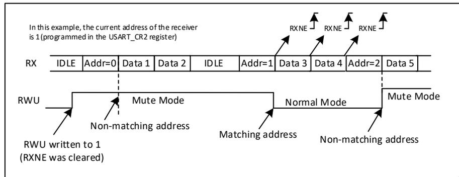
Figure 25-8 Silent mode with address tag detection
