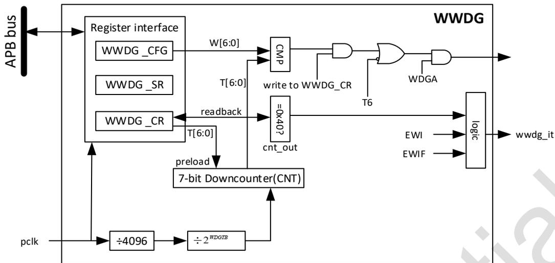
Figure 22-1 Window watchdog block diagram
