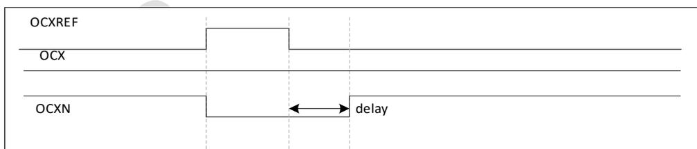
Figure 16-39 Dead-time waveforms with delay greater than the positive pulse.
