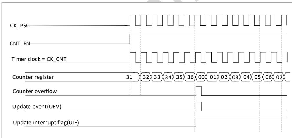
Figure 19-4 Counter timing diagram, internal clock divided by 1
