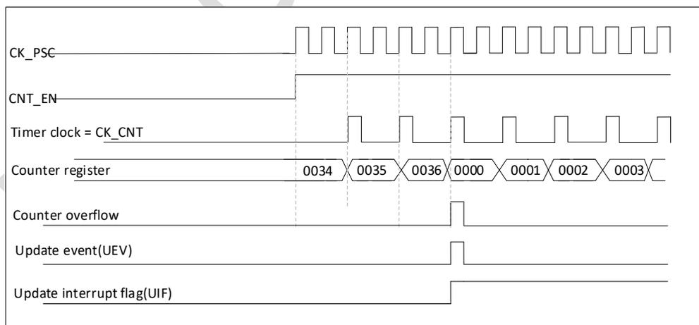
Figure 18-5 Counter timing diagram, internal clock divided by 2
