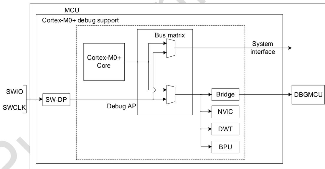
Figure 27-1 Block diagram of MCU debug support
