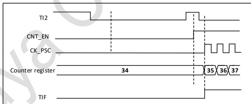
Figure 17-36 Control circuit in trigger mode
