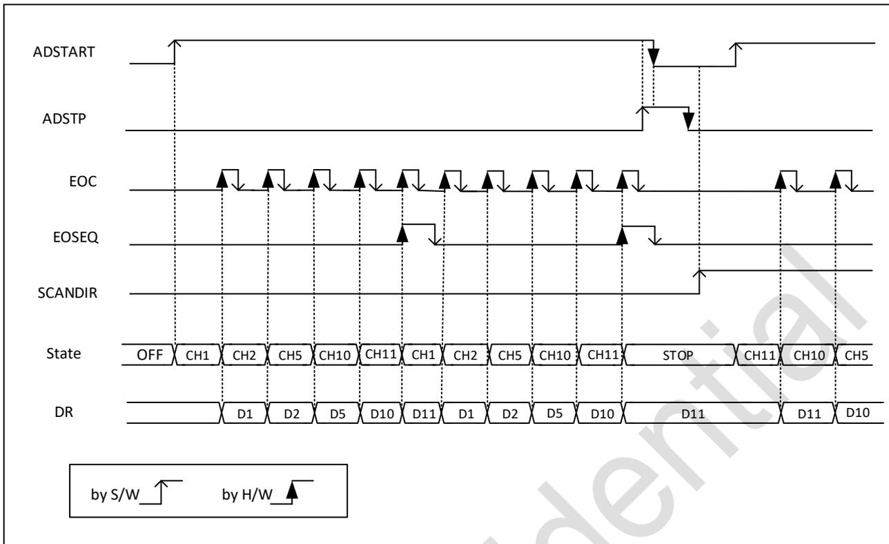
Figure 14-7 Continuous conversion of a sequence, software trigger
