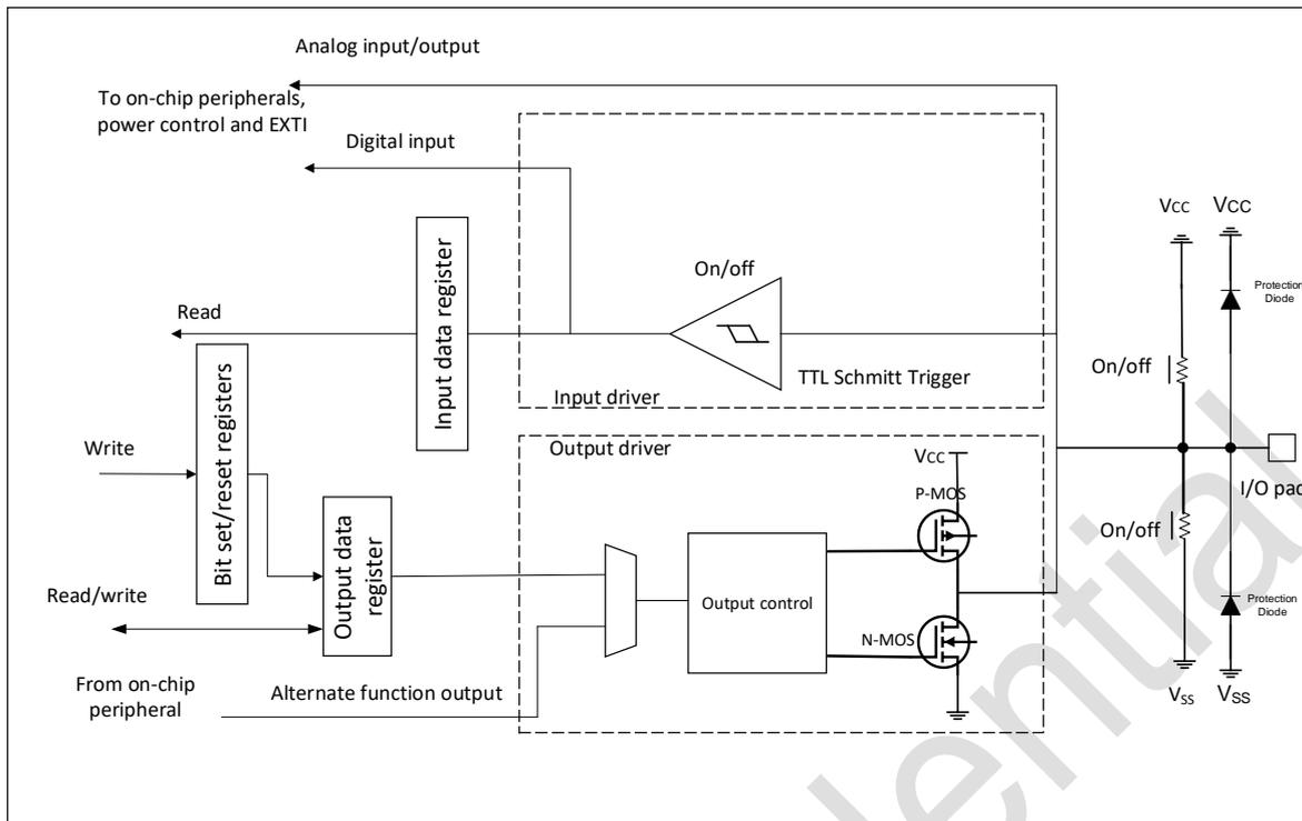
Figure 9-1 Basic structure of an I/O port bit
