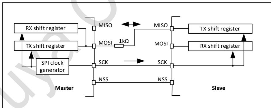
Figure 26-3 Half-duplex single master/slave application
