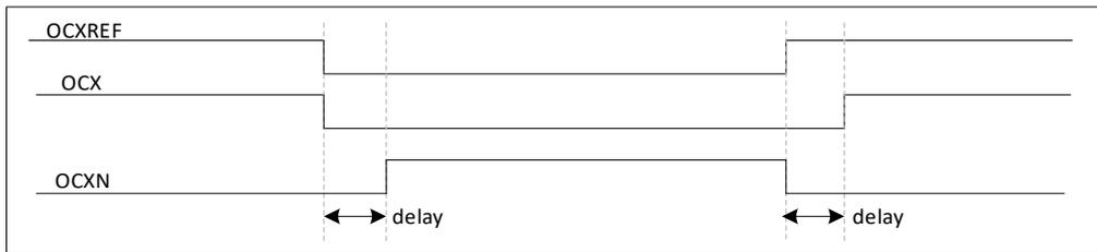
Figure 19-17 Complementary output with dead-time insertion
