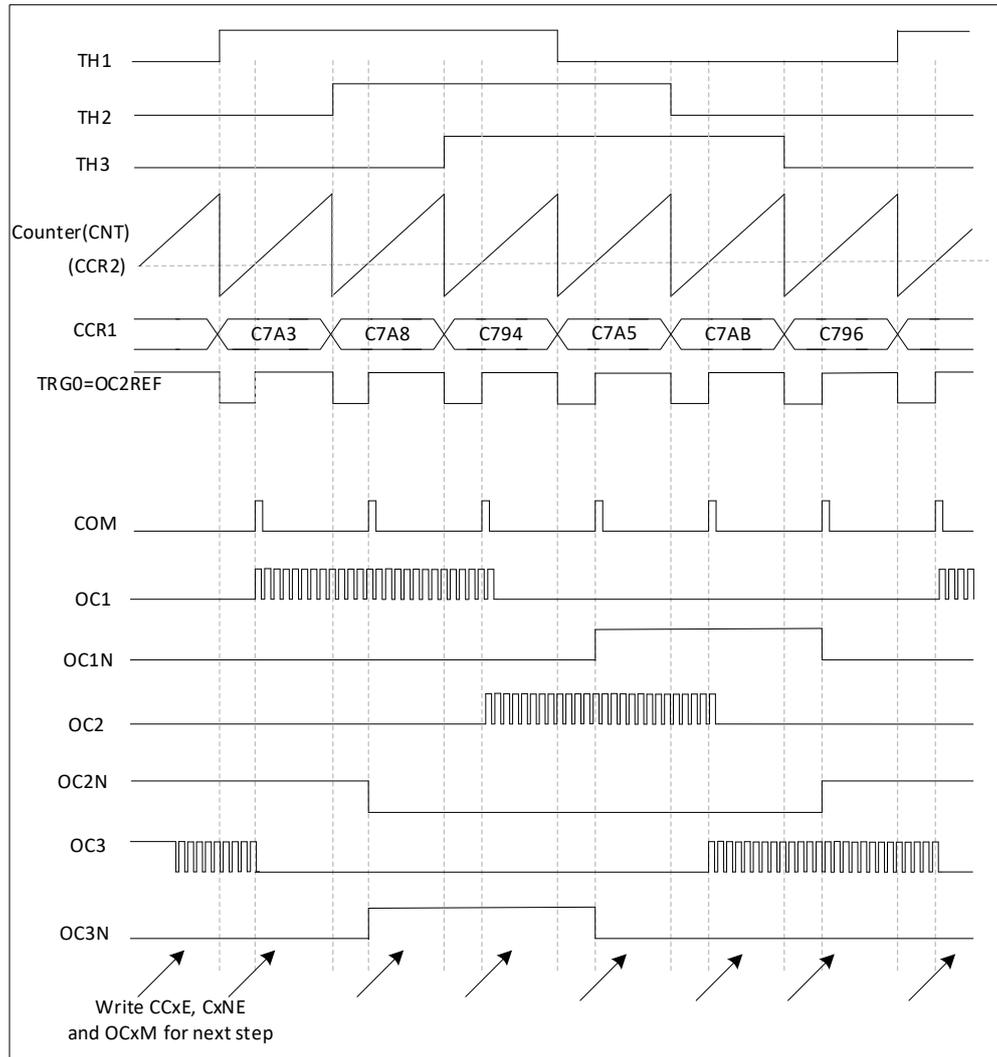
Figure 16-46 Example of Hall sensor interface
