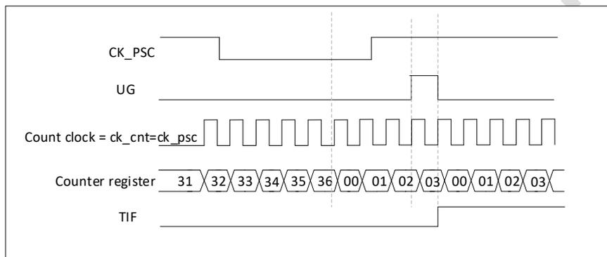
Figure 16-47 Control circuit in reset mode
