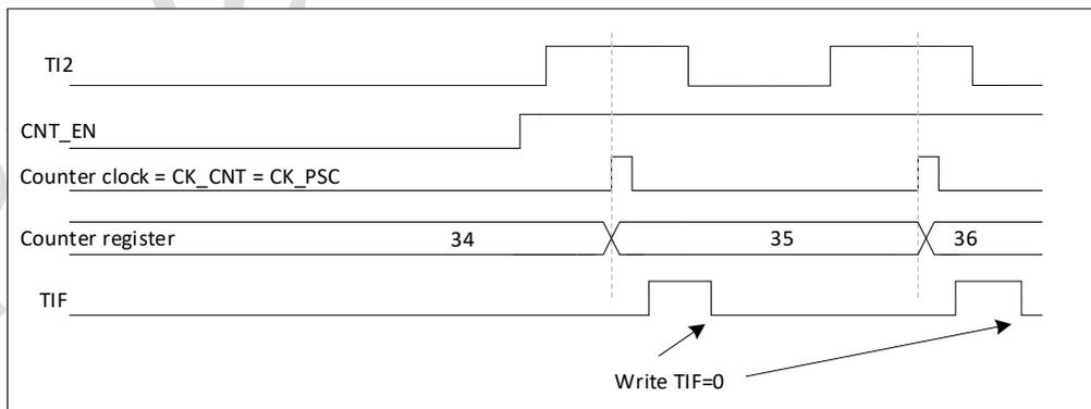
Figure 16-24 Control circuit in external clock mode 1
