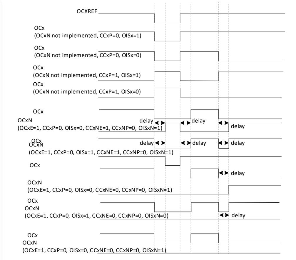
Figure 16-40 Output behavior in response to a break
