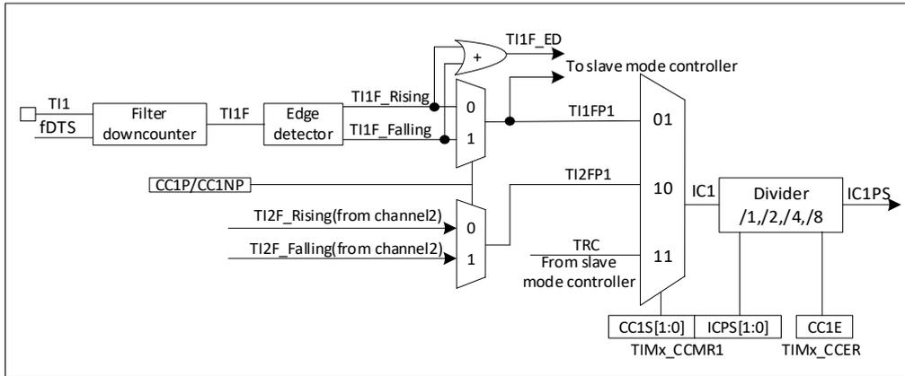
Figure 19-12 Capture/compare channel (example: channel 1 input stage)
