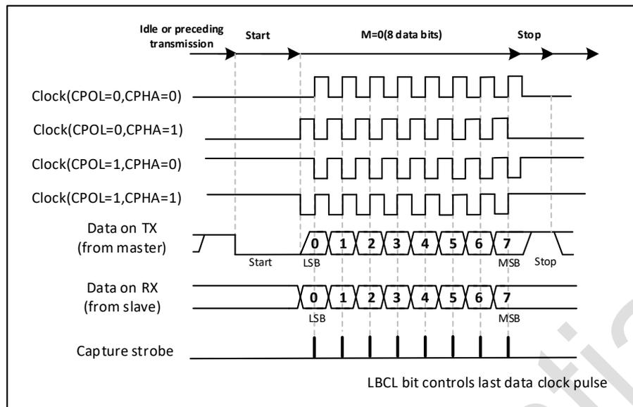
Figure 25-10 USART data clock timing example (M = 0)
