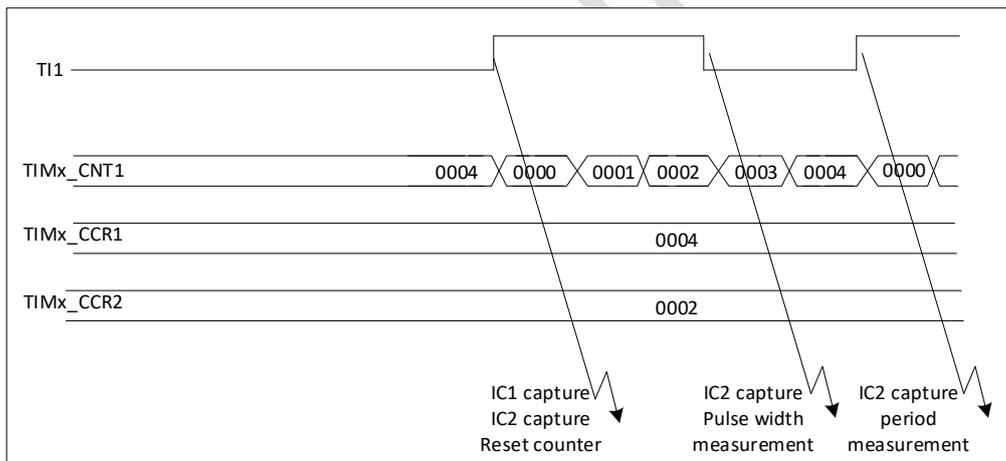
Figure 16-31 PWM input mode timing
