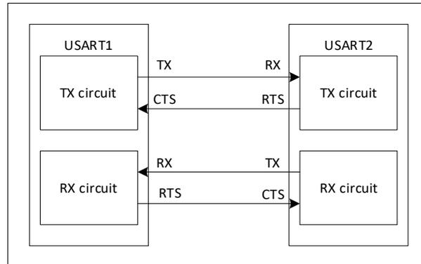
Figure 25-14 Hardware flow control between two USARTs
