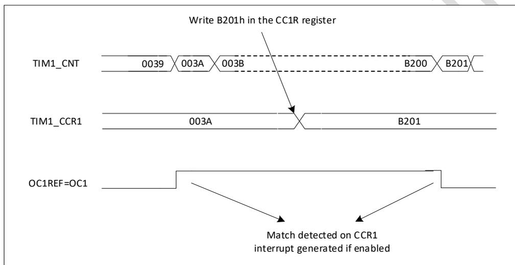
Figure 18-12 Output compare mode, toggle on OC1
