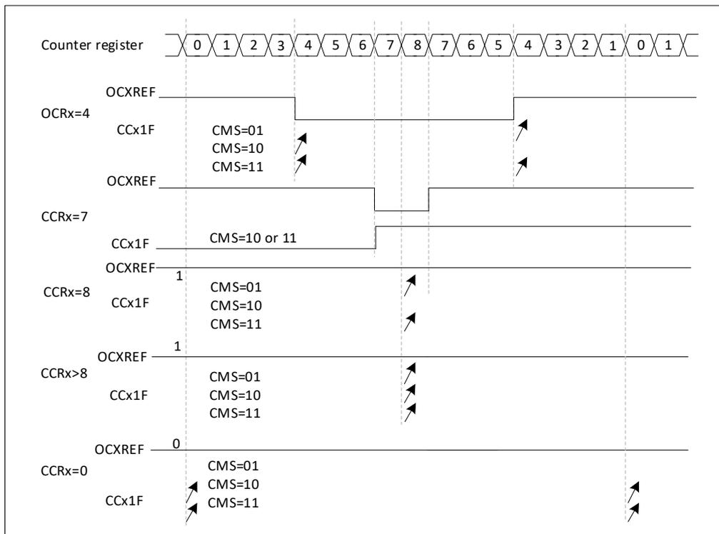
Figure 16-36 Center-aligned PWM waveforms (ARR = 8)
