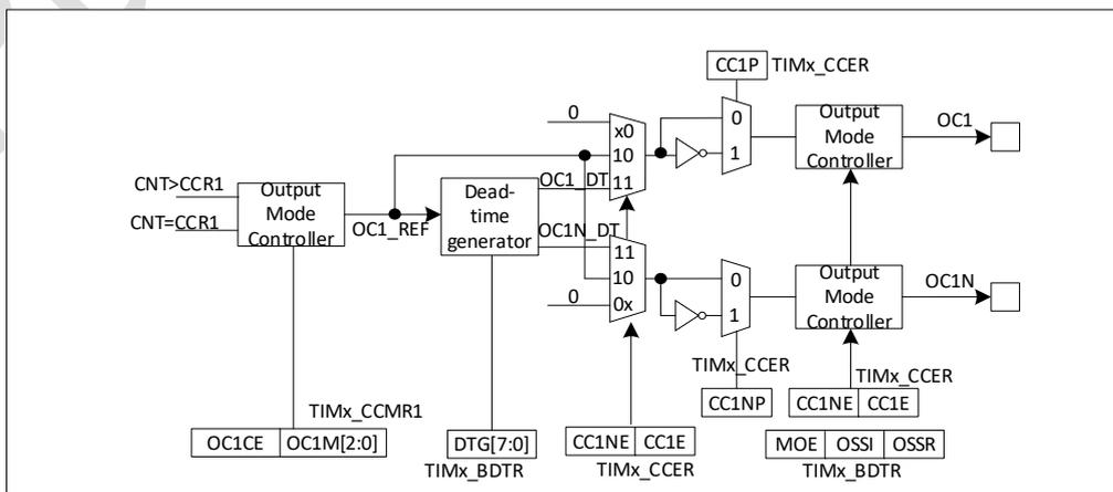
Figure 19-14 Output stage of capture/compare channel (channel 1)
