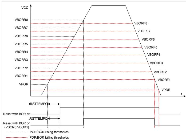
Figure 5-2 POR/PDR/BOR threshold
