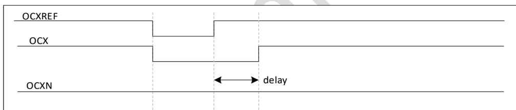
Figure 16-38 Dead-time waveforms with delay greater than the negative pulse.
