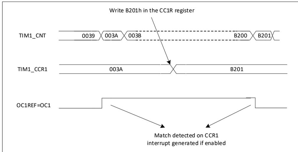
Figure 19-15 Output compare mode, toggle on OC1
