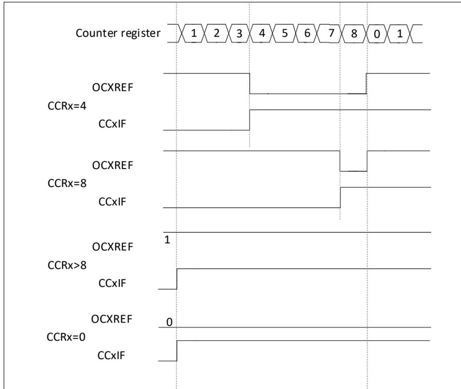
Figure 18-13 Edge-aligned PWM waveforms (ARR = 8)
