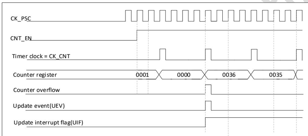
Figure 16-12 Counter timing diagram, internal clock divided by 4
