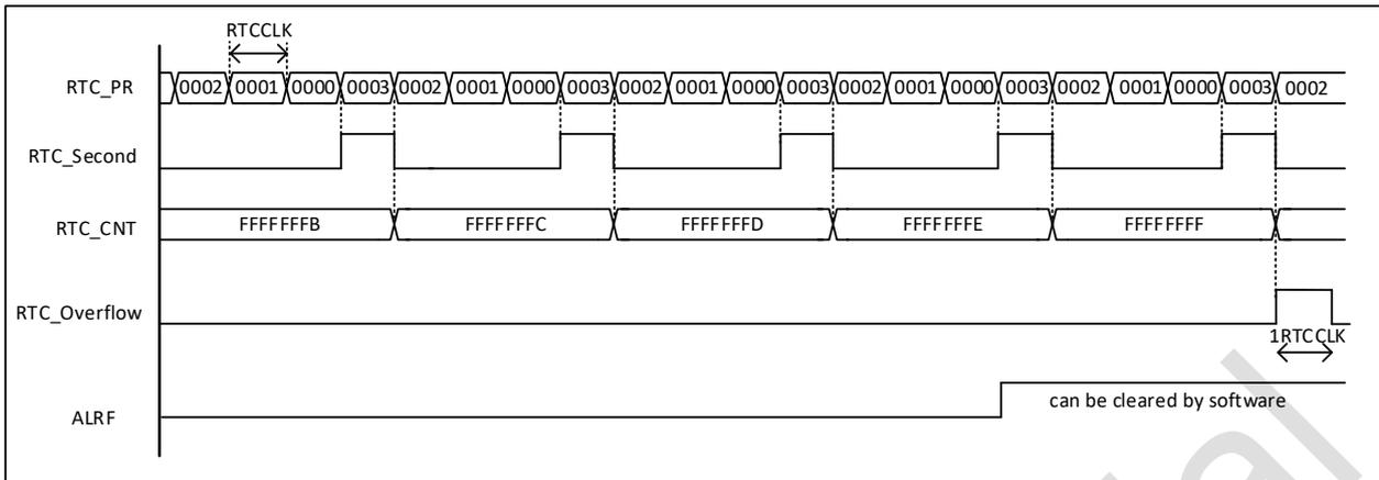
Figure 23-3 RTC overflow waveform example, PR = 0003
