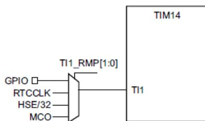
Figure 8-2 Frequency measurement with TIM14 in capture mode
