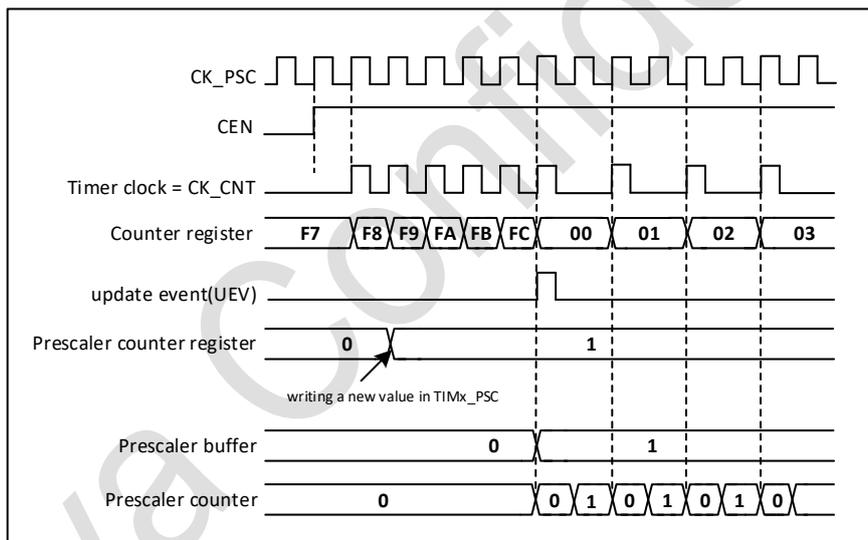
Figure 17-2 Counter timing diagram with prescaler division change from 1 to 2
