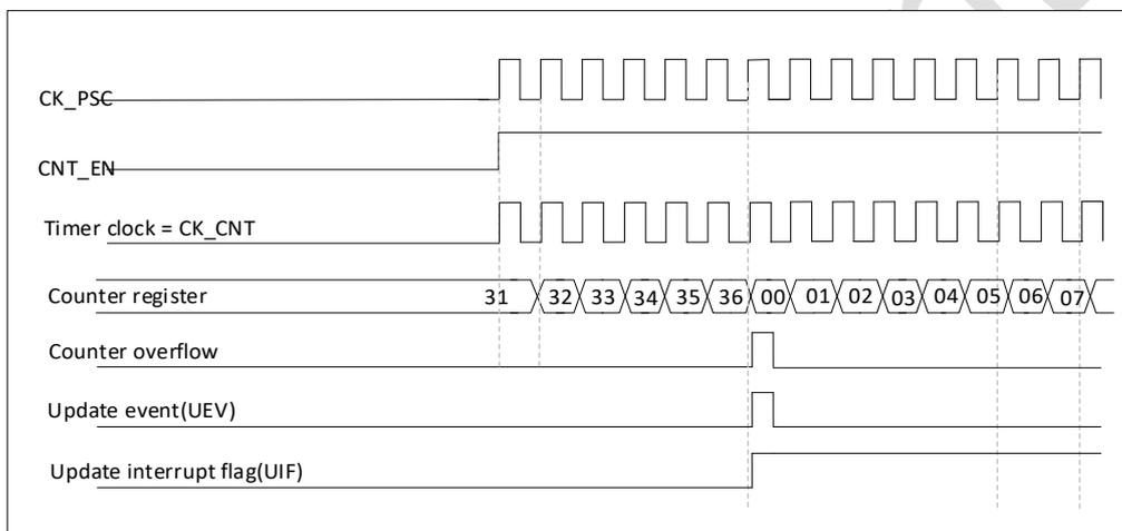
Figure 18-4 Counter timing diagram, internal clock divided by 1
