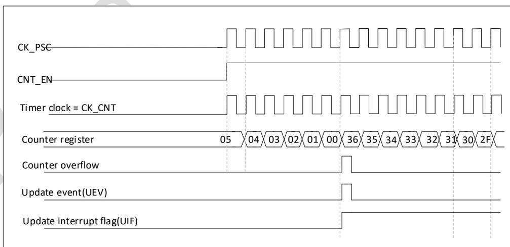
Figure 16-10 Counter timing diagram, internal clock divided by 1
